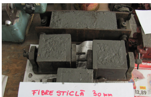
Fig. 6 – Glass reinforced concrete specimens – 30 mm fibre length.
