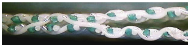
Fig. 10 – Cross-sectional view of a double layered woven filter fabric with stitched double layered selvages.
