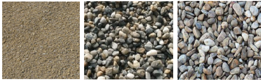
Fig. 2 – Aggregates in 3 sizes: 0–4 mm – size I, 4–8 mm – size II and 8–16mm – size III.
