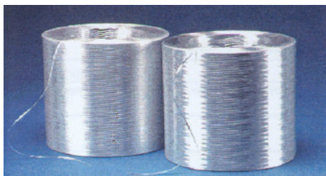
Fig. 3 – Glass roving –2400 tex ( www.vetrotextiles.com ).
