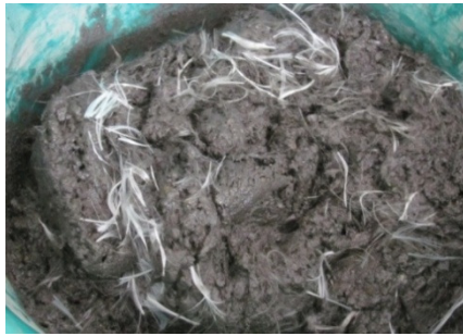
Fig. 8 – Mixing of fibres with concrete – non-uniform distribution – non-homogeneous mix.
