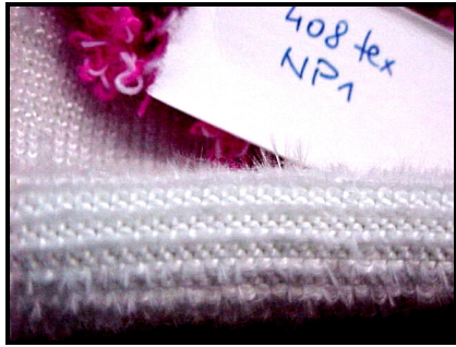
Fig. 5 – Aspect of the jersey fabric the knitted with NP1 = 10.5.
