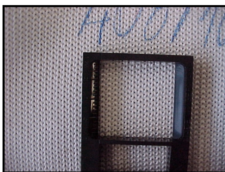
Fig. 1 – Aspect of a single jersey fabric, 408 tex.
