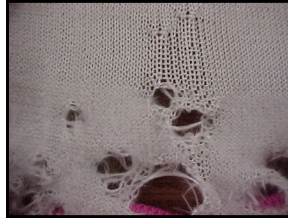
Fig. 6 – General aspect of a fabric knitted with the stitch length under inferior limit – 136 tex.
